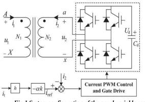
Fig 1 System configuration of the novel variable reactor
