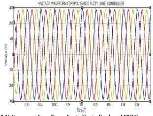
Fig 9 Voltage waveform Fuzzy Logic Controller based IPQC
